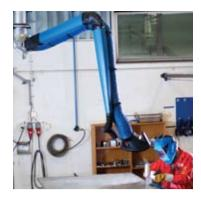
The Nederman range of low vacuum extraction arms covers a wide variety of applications. All arms are highly flexible, and simple to position, extend and retract. Different attachments are available for wall, ceiling or extension bracket mounting as well as a number of accessories, including hoods and dampers to improve efficiency.
