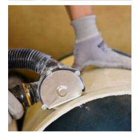
Nederman offers a range of high vacuum on-tool extraction kits for more than six hundred electric and pneumatic tools for cutting, grinding and sanding. The kits can be connected to both mobile vacuum units and stationary systems. The kits are available for the following brands of tools:
