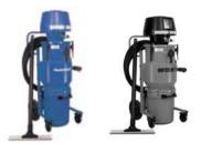
High capacity system for fine dust. Single container system with HEPA/Absolute filter. Efficient cyclonic pre-separation. Manual filter cleaning. Larger dust container as option. Ex version with ATEX approval: EX II 2 GD c IIC 60°C (140°F) (T6)
