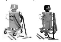
High capacity single container system for collection of coarse particles, as well as liquids and sludge. Allows transportation of material over long distances. Optional bottom drain valve for quick and simple discharge of liquids. Tippable container. With slots for forklift handling. Ex version with ATEX approval: EX II 2 GD c IIC 60°C (140°F) (T6)
