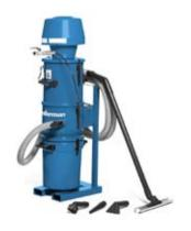
Single container system for fixed installation. Powerful vacuum unit suitable for recovery of liquids, dust and granulated material. Equipped with NVF filter, automatically cleaned at each system stop. Cyclonic discharge of the material into a container of 47 litres (12 gallons). Can be supplied with antistatic or conductive parts to avoid sparks from static electrical discharge. The unit is efficient for collecting greasy chips from lathes and drilling machines in a central suction system.
